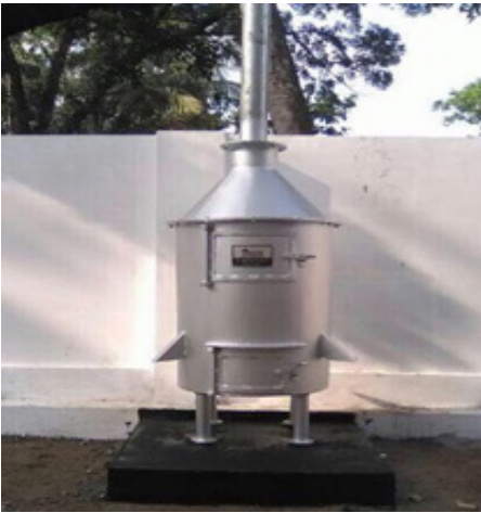
Fig 3: Solid Waste Incinerator: Capacity 25kg (Source: Indiamart, online shopping portal)
